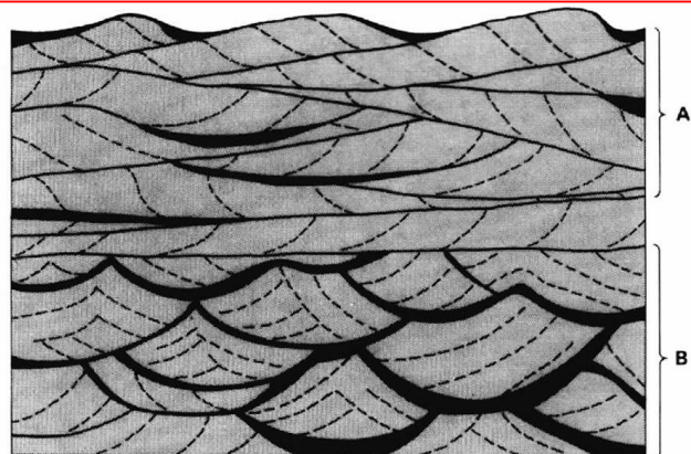
Figure 3.5 Flaser bedding: A, formed from current ripples; B, formed from oscillation ripples. The discrete mud lenses (black) in A and the sand-silt lenses in B often appear to 'float' and are referred to as 'biscuits'.
